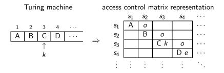
Turing machine with head over square 3 on tape, in state k and its representation as an access control matrix o is own right e is end right
